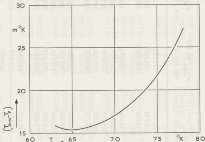
Fig. 3. Temperature differences between T_{\text{Arm.}} and T_p according to table IV. T_p is the temperature according to our final thermodynamic p - T relation given in table II.
