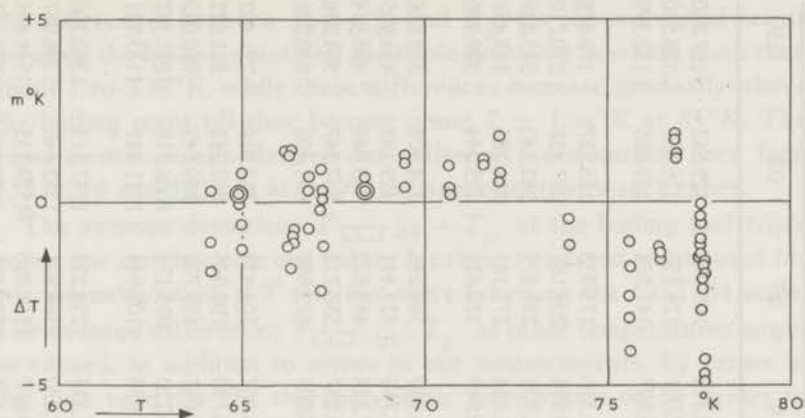
Fig. 13. Differences between temperatures T_{\text{CCT-64}} on the CCT-64 scale and temperatures T_p obtained from table II, chapter II, according to Armstrong's experimental data. \Delta T = T_{\text{CCT-64}} - T_p .
