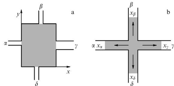
**Figure 1.** Four-terminal conductors; the disordered area is shaded. Reproduced from Ref. 10.
