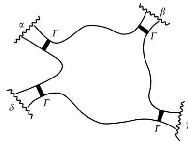
**Figure 3.** Chaotic cavity connected to four reservoirs via  $N$ -channel leads. Tunnel barriers of transparency  $\Gamma$  model the non-ideal coupling of the leads to the cavity. Reproduced from Ref. [30].
