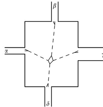
**Figure 2.** Typical electron trajectories, contributing to the exchange terms in the shot noise. Solid lines denote ballistic propagation (described by averaged single-particle Green’s function), and dashed lines denote diffusive propagation (described by the diffusion). Reproduced from Ref. 10.
