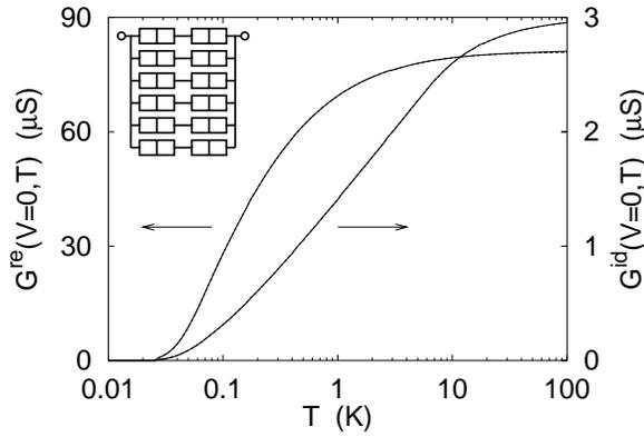
**Figure 2.** The zero bias conductance of a parallel array of 6 SDTJs (shown in the inset with sample structure given in the text) as a function of temperature for the *ideal* limit ( $G^{\text{id}}(T)$ ) and the *realistic* limit ( $G^{\text{re}}(T)$ ).
