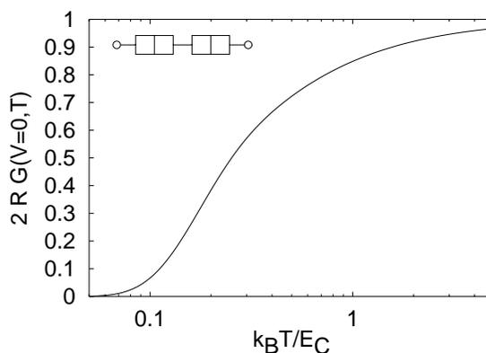
**Figure 1.** The universal functional dependence of the normalized conductance  $2RG(T)$  on the normalized temperature  $k_B T/E_C$  of a SDTJ (shown in the inset) at zero bias voltage  $V = 0$ .
