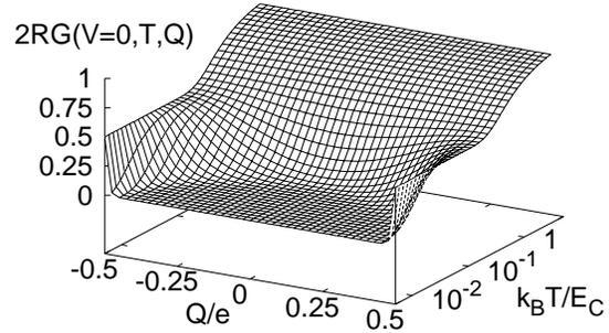
**Figure 3.** Effect of island offset charge  $Q$  on the universal functional dependence of  $2RG(T)$  on  $k_B T/E_C$  at zero bias voltage. The behaviour is periodic in  $Q$  with period  $e$ .
