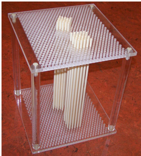
Figure 1.13. A photograph of a photonic crystal fragment from an ongoing experiment. The experiment is performed in the group of M. J. A. de Dood at the University of Leiden and aims, in particular, to test for 1/L scaling. Photograph by courtesy of M. J. A. de Dood.
