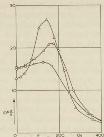
Fig. 4.16  $\text{CuNH}_4$ -tutton salt. The adiabatic susceptibility as a function of a longitudinal magnetic field at  $S = 0.2 R$ .
