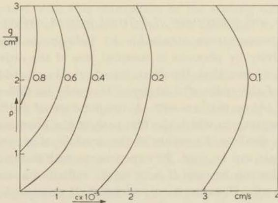
Fig. 3.8 The ratio of the energy transport from a CeMg-nitrate crystal to copper, using a glue and without it, as a function of the properties of the glue. The thermal resistance of the glue layer is described by  $l/L = 0.1$ .
