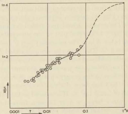
Fig. 2.3 The relation between entropy and absolute temperature of a solution of chromic ions in propyl alcohol ( $7.5 \times 10^{-4}$  mole/cm<sup>3</sup>). The dashed curve is calculated with  $\delta/k = 0.30^\circ$  K.
