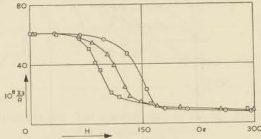
Fig. 4.10  $\text{CoNH}_4$ -tutton salt. The  $K_3$  susceptibility as a function of a longitudinal field.
