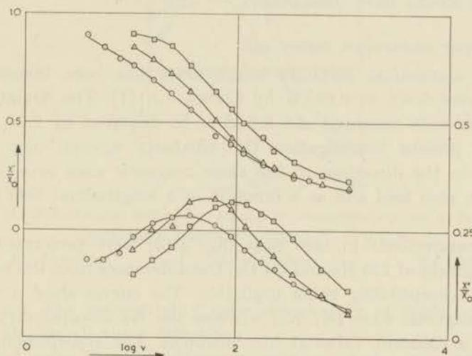
Fig. 4.14  $\text{CoNH}_4$ -tutton salt. Dispersion and absorption curves measured at  $S = 0.01 R$  with several amplitudes of the primary field.
