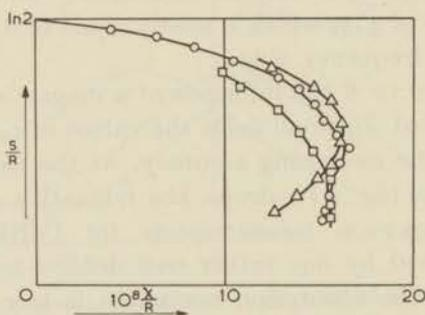
Fig. 4.15  $\text{CuNH}_4$ -tutton salt. The relation between susceptibility and entropy.  $\triangle$   $K_1$  direction  $\square$   $K_2$  direction  $\circ$   $K_3$  direction
