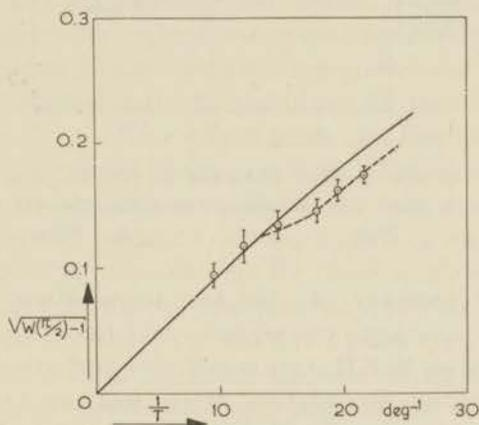
Fig. 6.7  $^{60}\text{Co}$  in  $\text{CoNH}_4$ -tutton salt. The relation between the  $\gamma$ -effect in the  $\text{K}_2$  direction and the absolute temperature. The solid line is calculated by means of  $A/k = 0.0200^\circ\text{K}$ .
