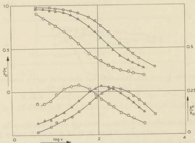
Fig. 4.13  $\text{CoNH}_4$ -tutton salt. Dispersion and absorption curves measured with a primary field amplitude of 0.05 Oe.
