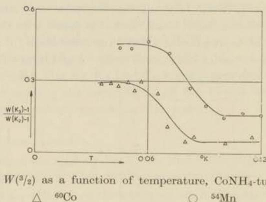
Fig. 6.6  $W^{(3/2)}$  as a function of temperature,  $\text{CoNH}_4$ -tutton salt.
