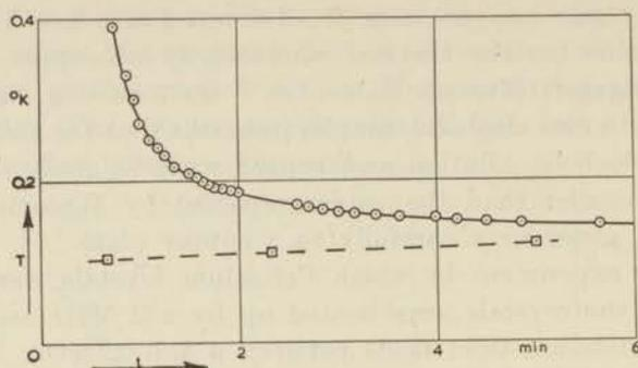
Fig. 3.3 A typical run. Temperatures of CrK-alum crystal and cooling solution as functions of time.
