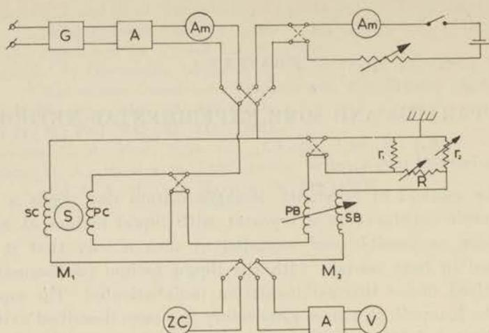
Fig. 1.1 The measuring bridge.
