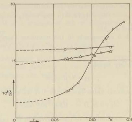
Fig. 5.2 MnNH<sub>4</sub>-tutton salt. The zero field susceptibilities as functions of temperature.
