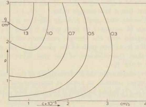
Fig. 3.7 The ratio of the heat flow from a perfect CeMg-nitrate crystal to copper, using a glue and without it, as a function of the density and the velocity of sound in the glue. The thermal resistance of the glue layer itself is neglected ( $l/L = 1$ ).
