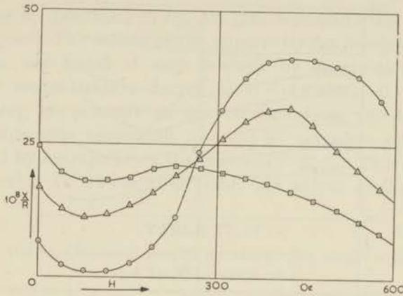
Fig. 4.5  $\text{MnNH}_4$ -tutton salt. The susceptibility in the  $K_1$  direction as a function of a longitudinal field.
