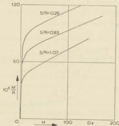
Fig. 4.8  $\text{MnNH}_4$ -tutton salt. Isentropic magnetization curves for a field in the  $K_3$  direction. The external fields have been corrected with  $H = H_e - (4\pi/3)M_v$ .
