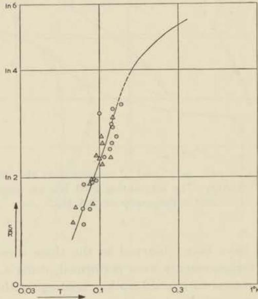
Fig. 4.4  $\text{MnNH}_4$ -tutton salt. The relation between absolute temperature and entropy. The solid line in the high entropy region has been derived from measurements of Cooke. The  $\chi'$  versus  $S$  relations with two different field amplitudes  $h_0$  are used as a thermometer.
