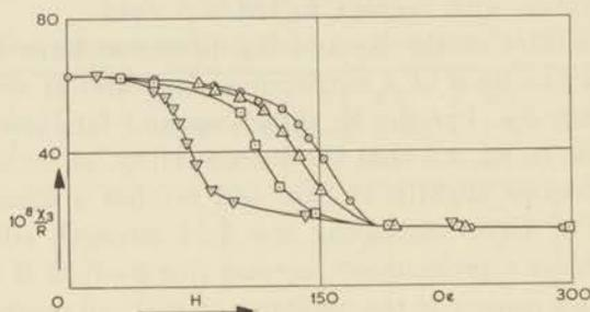
Fig. 4.7  $\text{MnNH}_4$ -tutton salt. The susceptibility in the  $K_3$  direction as a function of a longitudinal field.
