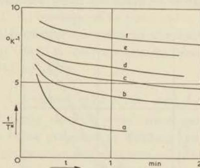
Fig. 2.4 Warming up curves obtained with a  $\text{Cr}(\text{NO}_3)_3 \cdot 9\text{H}_2\text{O}$  solution ( $2.5 \times 10^{-4}$  mole/cm<sup>3</sup>) after demagnetization from  $H = 2 \times 10^4$  Oe,  $T = 1^\circ\text{K}$ . The sample was kept at  $H = 1 \times 10^4$  Oe,  $T = 0.5^\circ\text{K}$  for a time increasing from curve a to curve f.
