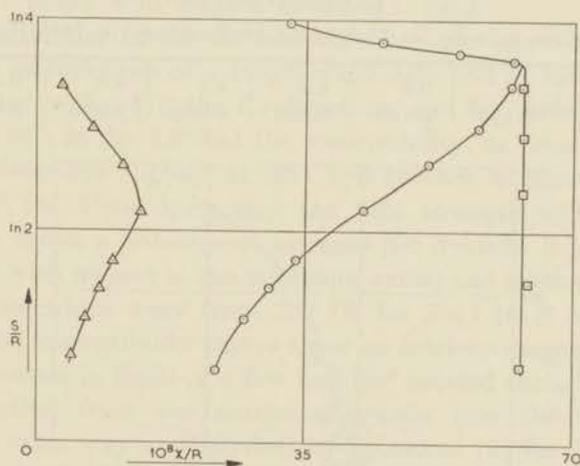
Fig. 4.3  $\text{MnNH}_4$ -tutton salt.  $\chi_0$ ,  $\chi'$  and  $\chi''$  measured in the direction of the  $K_3$  axis as functions of entropy. The alternating field has an amplitude of 0.05 Oe and a frequency of 225 Hz.
