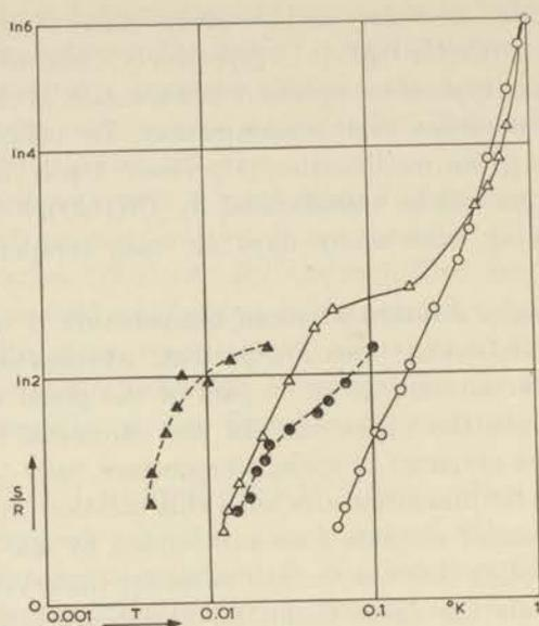
Fig. 2.6 The relation between entropy and  $T, T^*$  obtained with solutions of  $\text{FeCl}_3 \cdot 6\text{H}_2\text{O}$  in 1-propanol.
