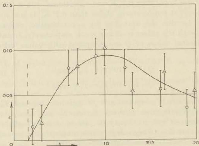
Fig. 3.5  $\gamma$ -anisotropy of  $^{60}\text{Co}$  in CeMg-nitrate as a function of time. The crystals were heated up at  $t = 1'30''$ .  $\epsilon = 0.08$  corresponds to  $T = 0.015^\circ \text{K}$ .
