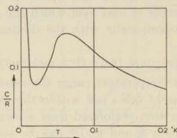
Fig. 2.8 The specific heat of a solution of  $\text{CuCl}_2 \cdot 2\text{H}_2\text{O}$  in 1-propanol ( $8.5 \times 10^{-4}$  mole/cm<sup>3</sup>) as a function of temperature.
