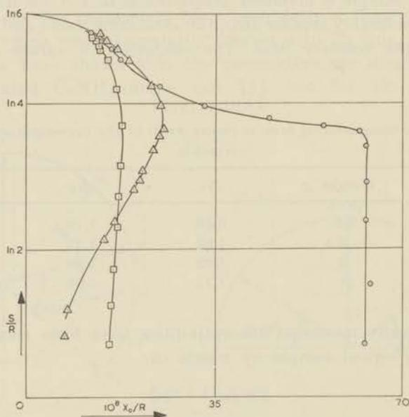
Fig. 4.2  $\text{MnNH}_4$ -tutton salt. The susceptibility measured in zero field as a function of entropy for the three magnetic axes.
