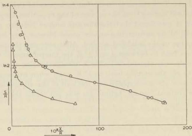
Fig. 2.2 Susceptibility versus entropy for a solution of chromic nitrate in propyl alcohol ( $7.5 \times 10^{-4}$  mole/cm<sup>3</sup>). A curve calculated with  $\delta/k = 0.30^\circ$  K is given in the high entropy region (dashed line).
