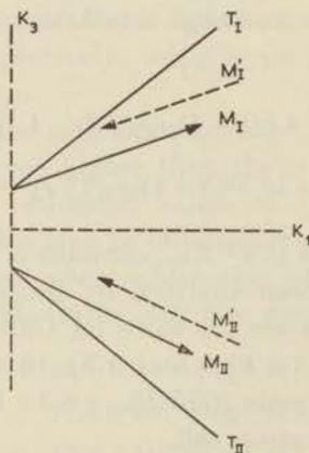
Fig. 5.3 The magnetic sublattices in  $\text{CuNH}_4$ -tutton salt below its transition temperature.
