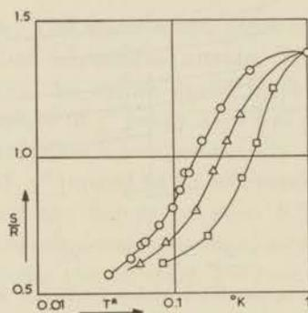
Fig. 2.5 The relation between entropy and magnetic temperature for three solutions of chromic ions in 1-propanol.
