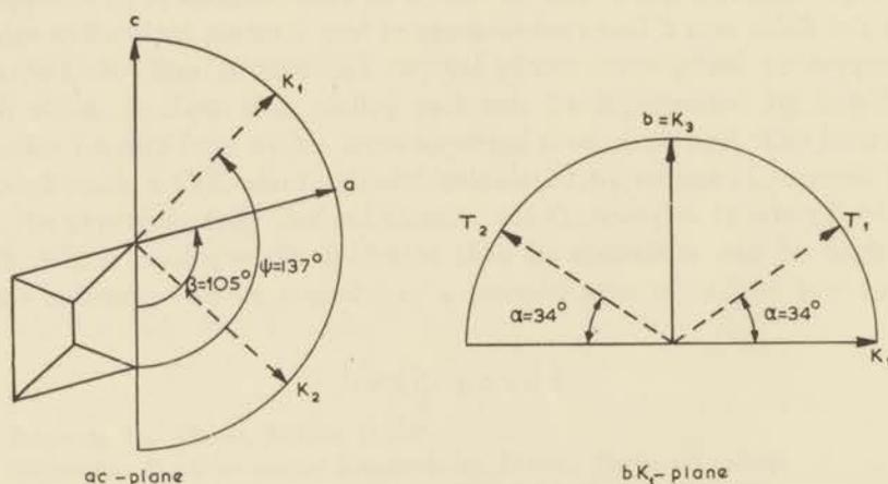
Fig. 4.1 Positions of magnetic susceptibility axes ( $K$ ) and tetragonal field axes ( $T$ ) with respect to the crystallographic axes in cobalt ammonium sulphate.
