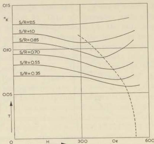
Fig. 4.6 The temperature variation during isentropic magnetization in antiferromagnetic  $\text{MnNH}_4$ -tutton salt. The dashed line represents the boundary of the magnetically ordered region.
