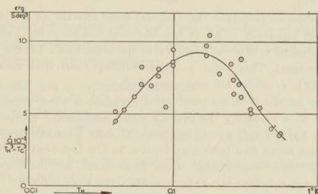
Fig. 3.4 Check of the formula  $\dot{Q} = B(T_h^3 - T_c^3)$ . If the formula were valid the  $\dot{Q}/(T_h^3 - T_c^3)$  versus  $T_h$  curve should be a horizontal line.
