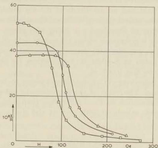
Fig. 4.19 CuK-tutton salt. The susceptibility as a function of a longitudinal field at  $S = 0.2 R$ .
