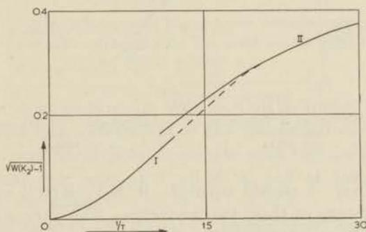
Fig. 6.5 The relation between  $\gamma$ -intensity in the  $K_2$  direction and the absolute temperature calculated by means of  $I = 3$ ,  $\mu/I = 1.1$  n.m.,  $A/k = 0.0104^\circ \text{K}$ ,  $D/k = -0.038^\circ \text{K}$  assuming:
