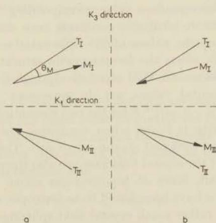
Fig. 5.1 Directions of the electron magnetic moments in  $\text{CoNH}_4$ -tutton salt in the magnetically ordered state.  $T_I$  and  $T_{II}$  represent the tetragonal field axes. There are two possibilities, *a* and *b*, for the antiferromagnetic structure.
