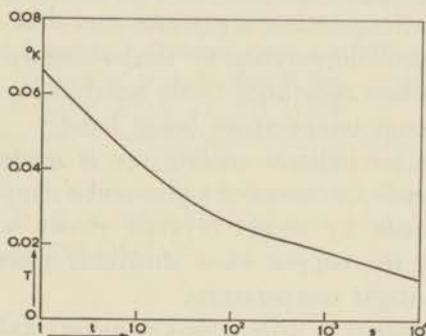
Fig. 3.9 The temperature of a cylindrical crystal as a function of time, the properties of the crystal being assumed as follows.
