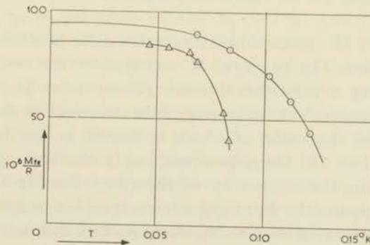
Fig. 4.9 The experimental values of the ferromagnetic saturation moment,  $M_{fe}$ , plotted *versus* temperature.
