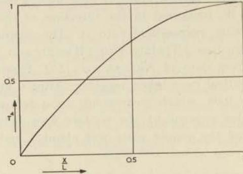
Fig. 3.6 Temperature distribution in a cylindrical CrK-alum crystal of length  $L$ , which is cooled at  $x = 0$ . The heat flow through each  $\text{cm}^2$  cross-section of the crystal is given in arbitrary units by the derivatives of the curve.
