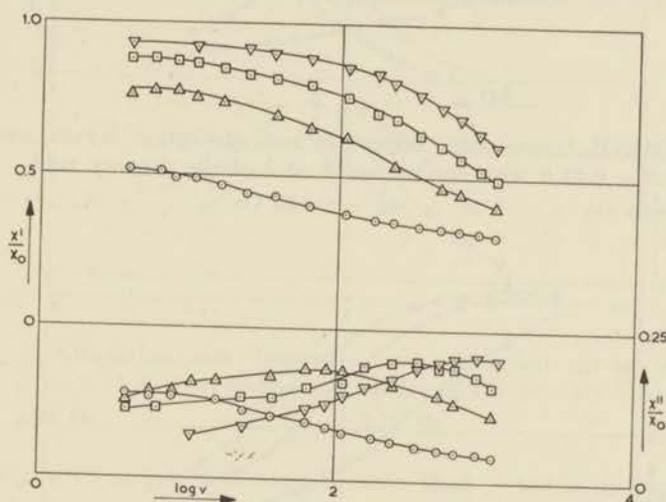
Fig. 4.11  $\text{MnNH}_4$ -tutton salt. Dispersion and absorption curves measured with a primary field amplitude of 0.05 Oe.
