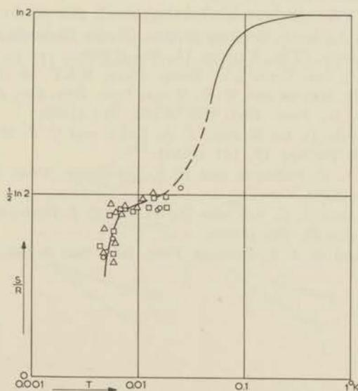
Fig. 4.20 CuK-tutton salt. The relation between absolute temperature and entropy. The solid line, given in the high temperature region, is derived from data of Garrett.
